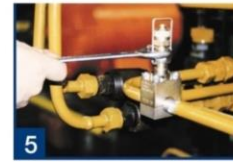
5 screw the valve to the right until it stops then screw it to the left
