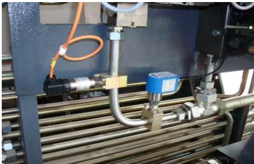
Picture 2: Pipe measuring point serv-Clip -1 with pressure sensor (threaded coupling G 1/4")
