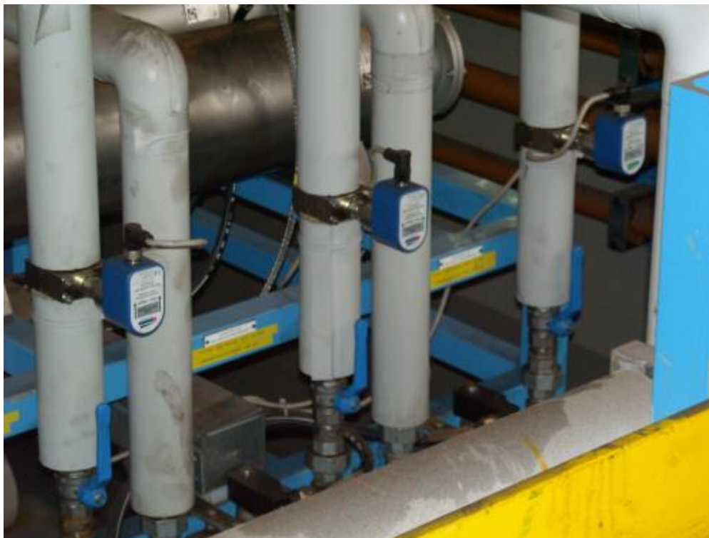
Picture 4: Control of a lubrication oil line with flow rate sensors fluid-Check and serv-Clip -2 at a continuous pickling line.
