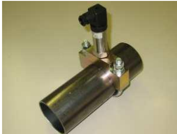
Picture 5: Temperature and pressure sensor with serv-Clip -2
